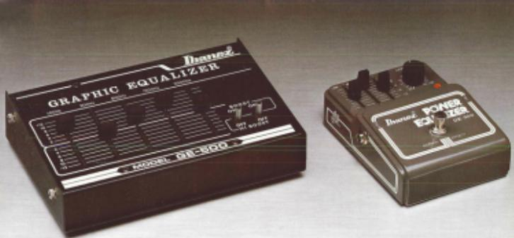
The Ibanez GE-500 is a simple, easy-to-use, moderately priced instrument equalizer suitable for almost any use. It covers five bands within the frequency response of most instruments.
