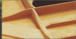
Scalloping, the technique of contouring the interior braces of the top, allows for maximum vibration while maintaining maximum strength.
