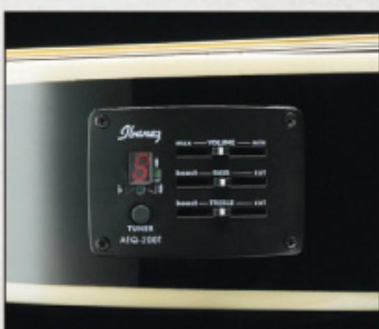
The Ibanez AEQ200T, which has 2-band tone control with onboard tuner, is optimized for use with Ibanez Under Saddle Pickups. 7 segment LED display enables you to tune, wherever and whenever necessary.
