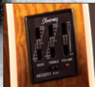
TCY20 models feature an Ibanez piezo pickup and Ibanez AEQ201 preamp with 2-band EQ.
