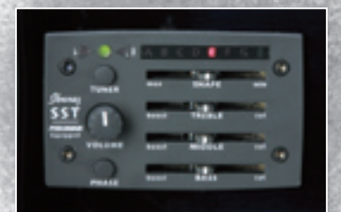
Fishman® Sonicore Pickup & Ibanez AEQ-SST Shape Shifter™ Preamp with Onboard Tuner
