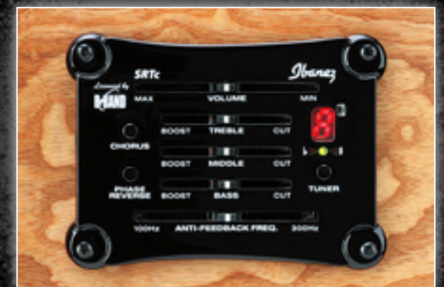
Ibanez SRTc Preamp with Chorus, Phase Reverse with Anti-Feedback Frequency and Onboard Tuner
