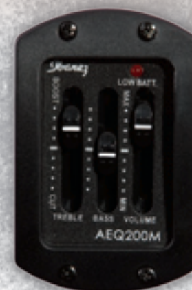
Ibanez AP2 magnetic soundhole pickup and AEQ200M preamp with 2-band EQ on TCM50VBS.
