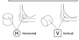
The Body Stoppers can be positioned in either a horizontal or vertical orientation. Select whichever position best accommodates the instrument being stored in the case.
