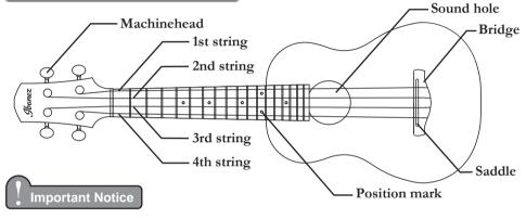
Ukuleles are primarily made of wood. Wood will remain stable over a long period of time if it is kept at appropriate temperatures and humidity levels, but will swell or shrink if used or stored in an environment of extremely high or low temperatures, or humidity levels. For a long lifetime of your ukulele, we recommend you to avoid keeping it in such a severe environment.
