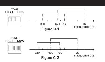
B. The Twin Peaks wah pedal has two sweepable range modes. (See Figure C-1 and C-2)
