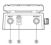
6. Ext. DC Input: Be sure to use a center negative external DC power supply (AC/DC adapter etc.)
