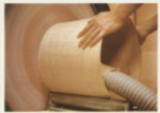
Tama Fibrestar shells are made by the "hand lay up" procedure, where fibreglass cloth is placed by hand in a rotating mold. The mold is then spun at a high speed while the resin is poured, resulting in a very uniform thickness. The fibreglass/resin shell is then heat cured in the spinning mold and is removed as a complete shell.
