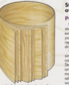
As each of the nine Starclassic plies are precision milled to a 0.3mm thickness (Starclassic Maple), the wood must be hand-selected plies for optimum density and quality. These plies are each cross-laminated at a 90 degree angle for greater strength.
