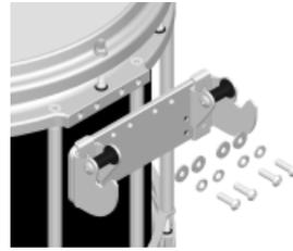
Attach the carrier attachment to the snare drum by tightening with an "L" wrench. It is advisable to use glue to prevent screws from becoming loose.
