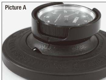
2. Place the Tension Watch on a level surface such as glass or a mirror and set the needle to "0" on the dial by rotating the dial inside the dial cover. (Picture B)
